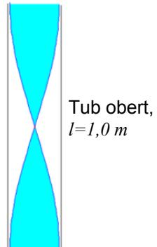
**0.2 p**  $v_0 = \lambda f_0 \Rightarrow f_0 = \frac{v_0}{\lambda_0} = \frac{343,0}{2,0} = 171,5 \text{ Hz}$
